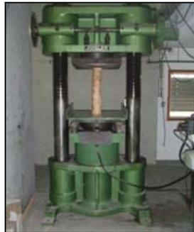
***Figure 8: Compression test***
