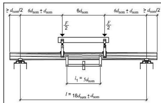
**Figure 7: Schematic representation of the bending test**
