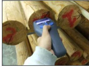
*Figure 9: Non-destructive test with MTG*
