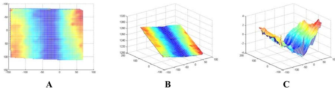
**Figure 5: The projected surface of the wooden sample, a) camera view, b) bottom side view, c) difference of the projected surface from the flat surface. The camera is placed in the origin  $[0,0,0]$ , units are in mm**
