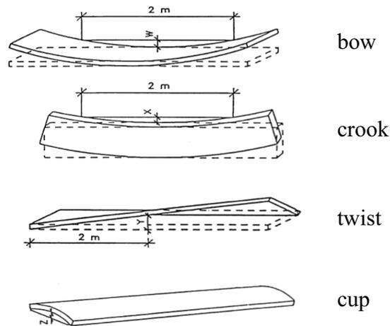
**Figure 2: Distortion of wooden boards**
