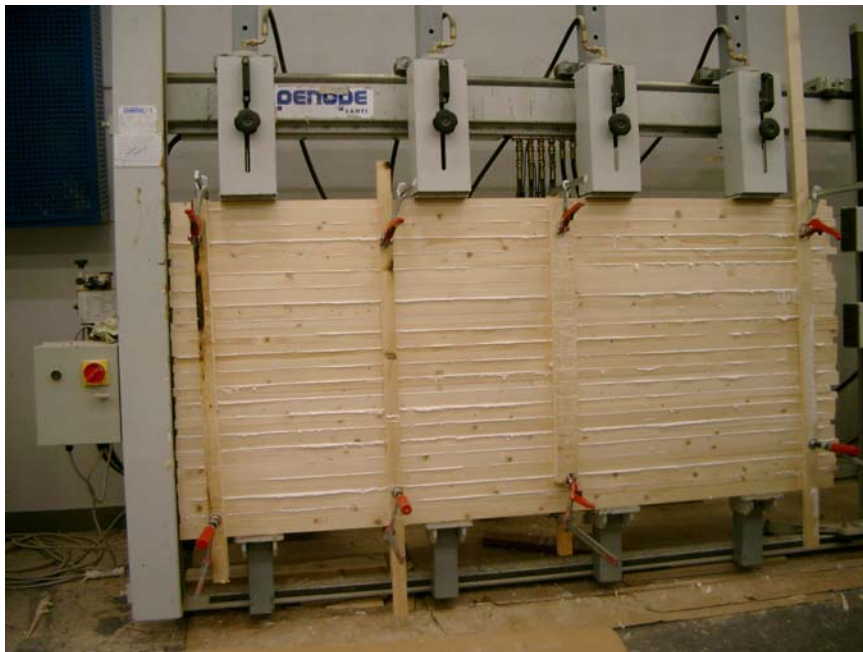
Figure 2: The vertical press used in the tests. Photo: Keijo Heikkilä
