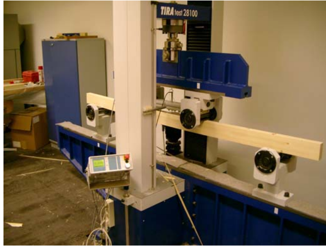
Figure 3: TIRA test 28100 material testing device with the external extensionmeter in the middle of the beam. Photo: Keijo Heikkilä
