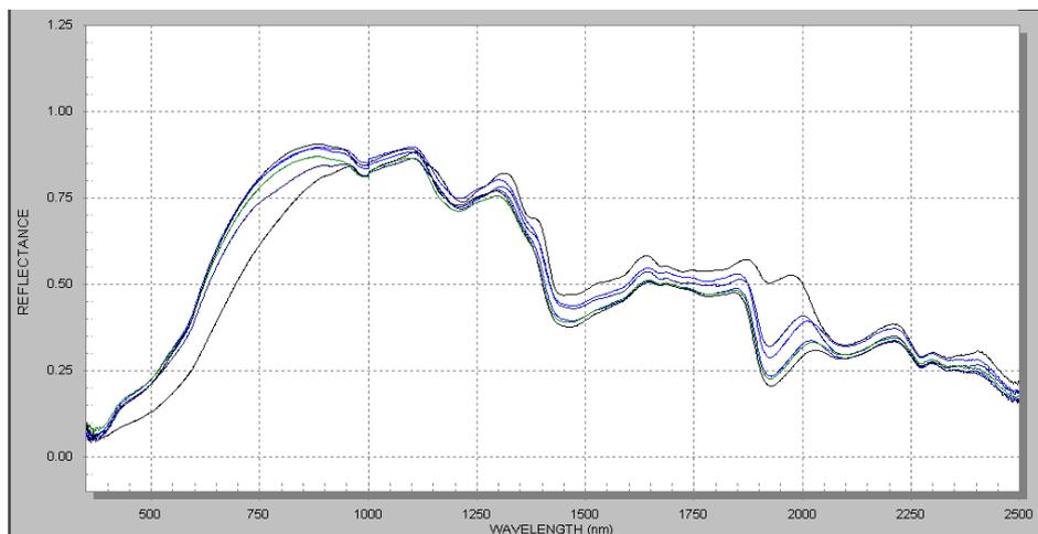
**Figure 1: NIR spectra at various moisture contents**
