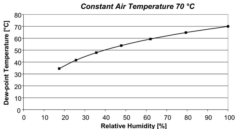
**Figure 1: Dew-point temperature as function of relative humidity**
