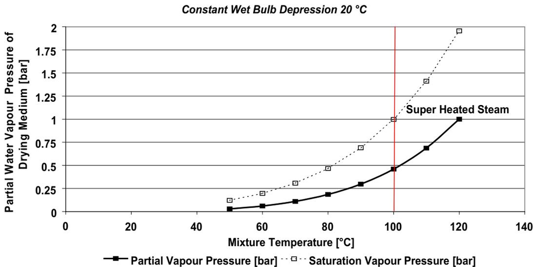
**Figure 2: Water vapour pressure of drying medium (air-steam)**
