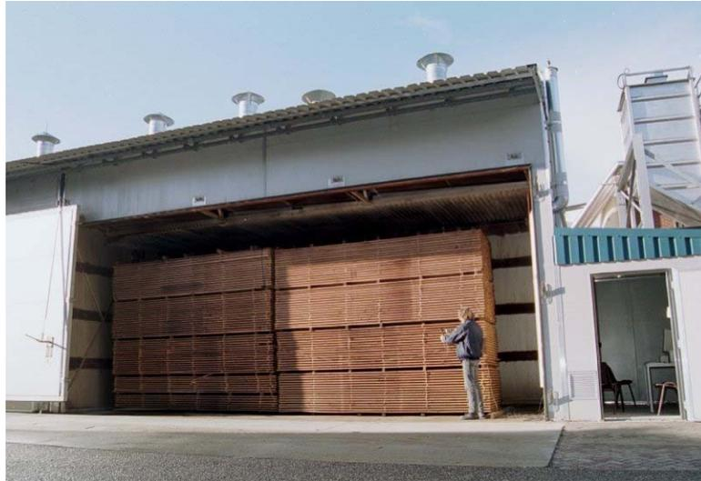
**Figure 4: Industrial kiln for super-heated steam drying**
