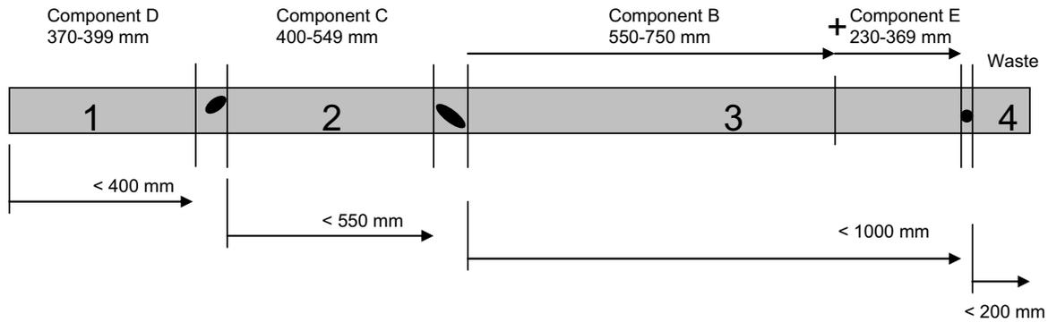
**Figure 3: Illustration for cross cut kerfs along a sawn board with four clear board zones**
