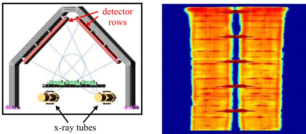
**Figure 1: Delineation of a two-source x-ray scanner (here a Microtec Tomolog<sup>®</sup>) and the image of a log produced by such a scanner**
