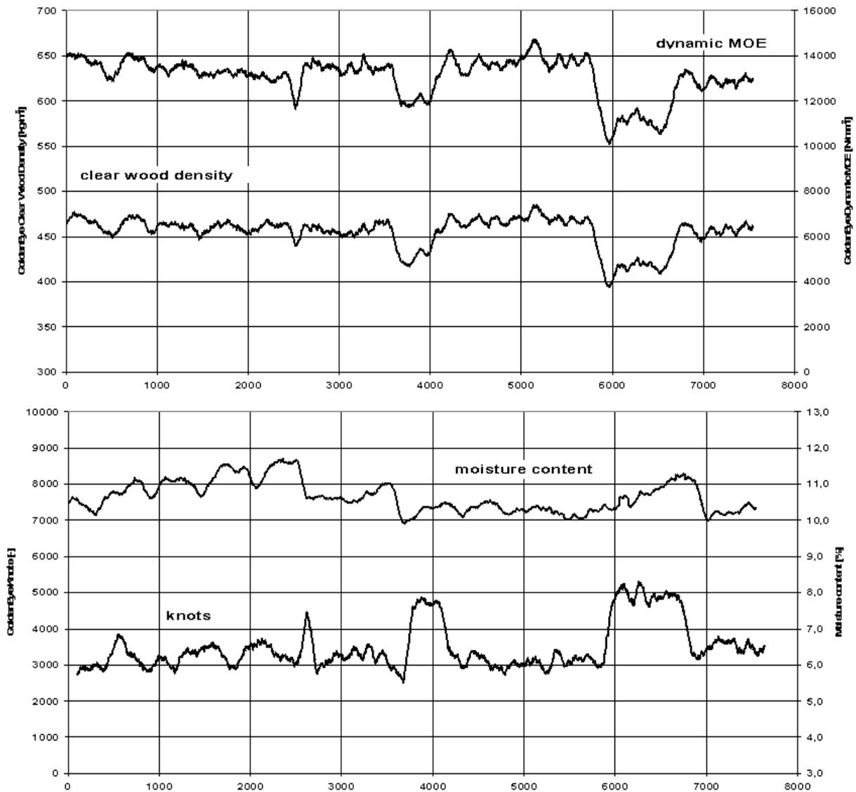
**Figure 1: Quality shifts observed by GoldenEye-706 within 4 hours of production of spruce 44x88 (mean values calculated with a sliding window of 100 pieces for clear wood density, dynamic MOE, knots and moisture content)**
