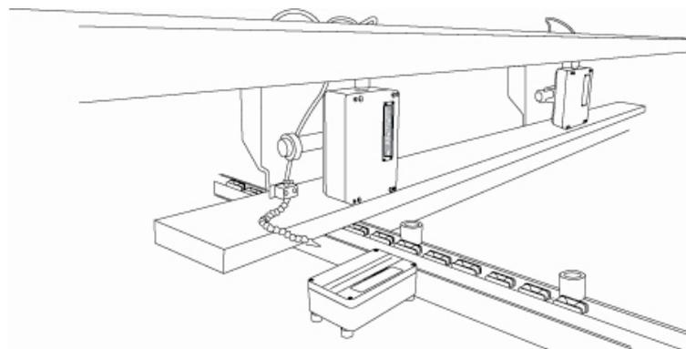
**Figure 2: DENSCAN (measuring density based on X-ray technology on transverse transport)**
