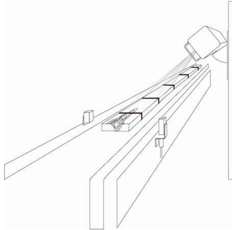
**Figure 7: CURVESCAN (warp measurement unit in longitudinal transport)**
