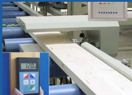
Figure 1: In-line MC measuring system and hand-held MC meter
