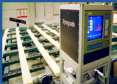
Figure 2: In-line strength grading
